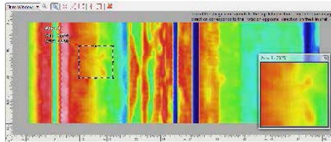
The IRT KilnMonitor® allows operators to select their own color palette and temperature range of interest. They can read information about temperature at a specific spot, position of the spot, brick thickness, coating thickness, etc. The software also allows them to zoom in on a specific area in a separate window.
