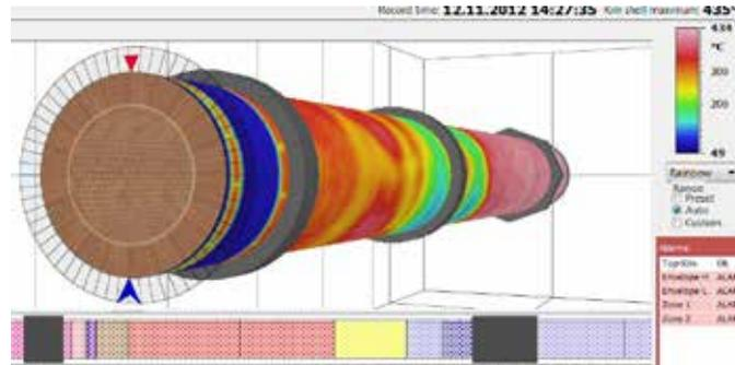
This viewing mode virtually cuts the kiln at some position and shows the kiln interior (bricks and coating).
