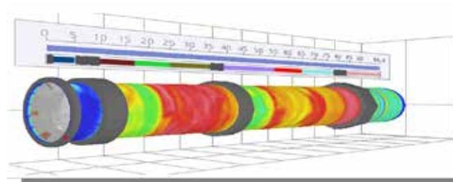
This view presents the kiln "pipe" temperature on the surface as a thermal image. The kiln is rotating in real speed.
