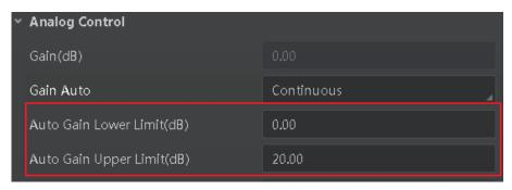
Figure 11-20 Set Gain under Once or Continuous Mode
