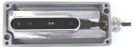
The mount guarantees good heat dissipation
