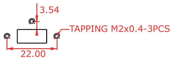
Figure 1: Threading hole dimensions for USB connectors
